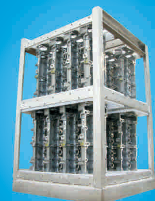
Fixturing to process fully machined parts
